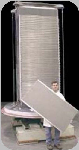
Individual fuel cell & 350 kW fuel cell stack
