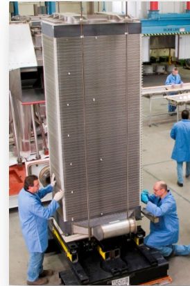
400 components are used to build one 350 kW fuel cell stack
