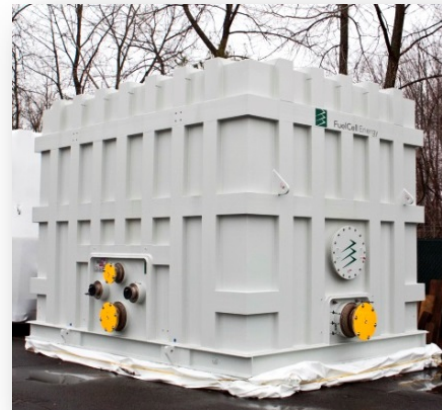
The stacks are enclosed, creating the fuel cell module
