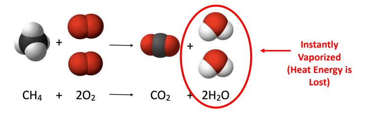
Condensing Heat Recovery Reduces This Loss!
