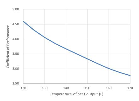
Graph shows representative values for the COP of a heat pump driven with a heat source of 50°F for a range of heat output temperatures.
