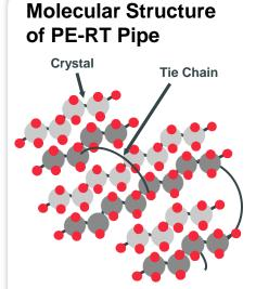
Tie chains in the high molecular weight fraction connect the crystalline structure in the polymer, which toughens the material and gives it superior strength at high temperatures.
