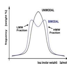
Dual reactors (versus one) are utilized to create PE resin with bimodal (two) molecular weight peaks – providing the extruded pipe with the properties required to perform in raised temperature and oxidative environments.
