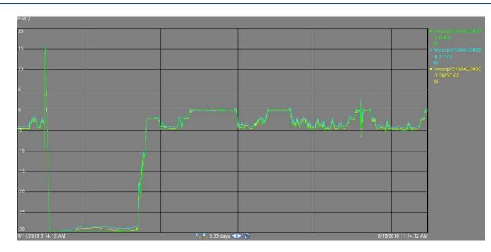
Three Guided Wave Radar Tracking Within 0.5 Inch
