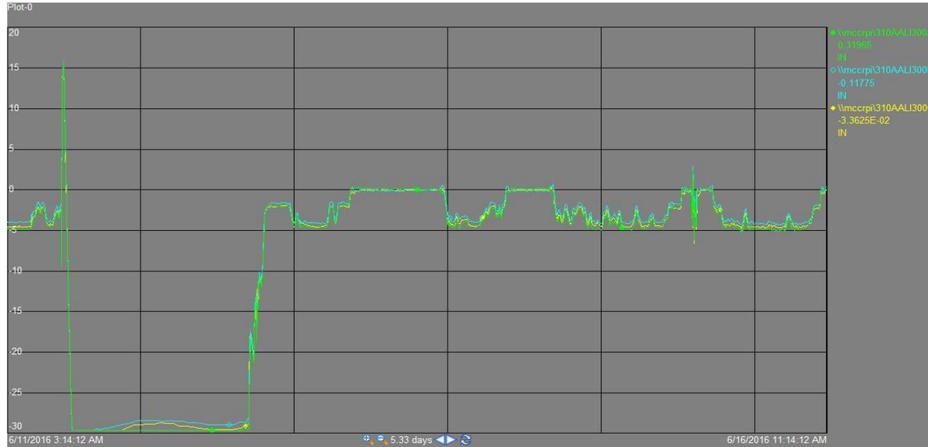
Three Guided Wave Radar Tracking Within 0.5 Inch
