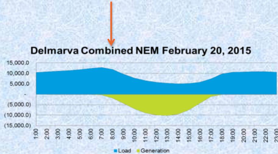
3. Output Profile – the output profile doesn't match the load profile of the premise or aggregate system load (shown)
