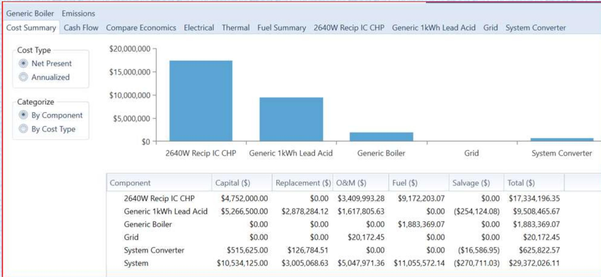
**Conclusion: Net Present Cost for 15 year for the system is \$29.3 million from capital costs of CHP and battery. Highest expenses for this comes from fuel for CHP and O&M as in the break-down of expenses in the table.**
