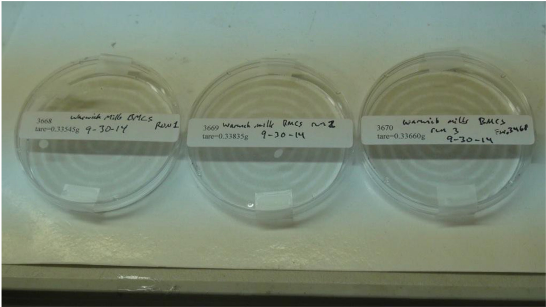
Fig. 7 Filters after emission test. Warwick Mills, 2014
