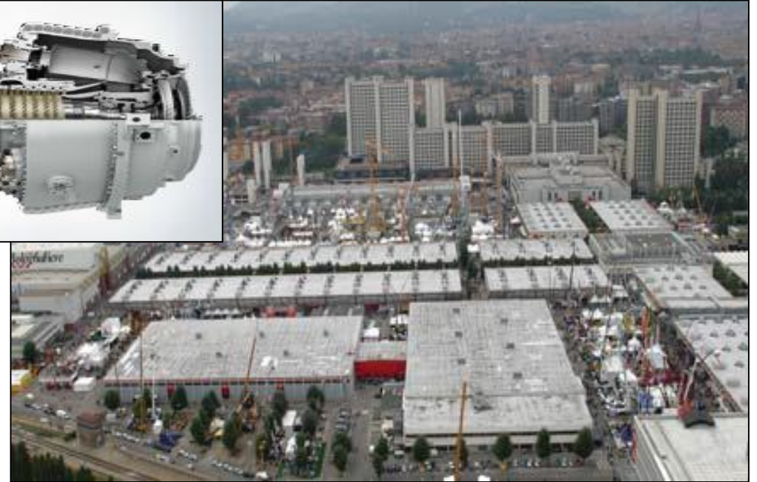
CHP plant at BolognaFiere Exhibition Center (Italy) SGT-100 Gas Turbine 4.7 MW(e) and steam for heating and air conditioning
